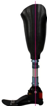
For the correct A/P position of the foot, position the socket's reference line (socket – ankle) approximately 0-5 mm posterior of the socket position.
