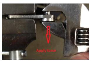
Use a vise (a rag is recommended to protect hinge surfaces) to secure one leaf of the hinge, and then apply force with a crescent wrench to bend to shape
