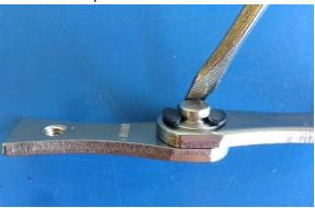
Set the hinge on a table vertically, then use a narrow screw driver to pull out the c-clip downward. A rubber mat or card board is recommended to put on top of the table to avoid damage
