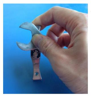
Use the curvy part of the wrench to check the clip is sitting right in the groove by pushing down
